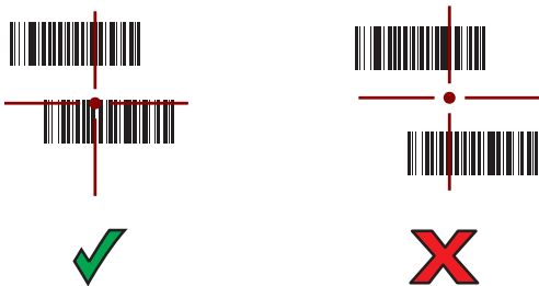
Figure 125 RS507/RS507X Pick List Mode with Multiple Barcodes in Aiming Pattern
