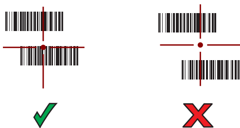
Figure 128 RS6000 Pick List Mode with Multiple Barcodes in Aiming Pattern
