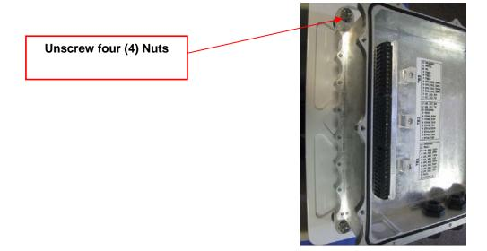
L) Remove the back cover from the WhereTrack Module by unscrewing 29 screws.
