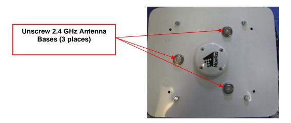
F) Unscrew the cable from the GPS Antenna then remove the GPS Antenna by unscrewing four (4) screws.
