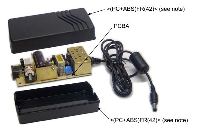
Note: Unless otherwise marked, the power supply enclosure is constructed with >(PC+ABS)FR(42)<
