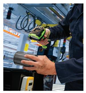
DS3600-DP and DS3600-DPA models bring the lightningfast capture of virtually every direct part mark to aerospace, automotive and other manufacturing plants where end-to-end traceability of product components is required.
