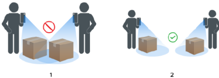
Figure 9 Dimensioning with Multiple Devices
