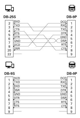
Interconnecting to DCE Devices – When the printer is connected via its RS-232 interface to data communication equipment (DCE) such as a modem, a STANDARD RS-232 (straight-through) interface cable must be used.
