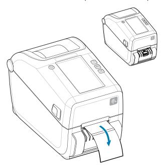
**2.** Lift the liner over the top of the printer. Pull the gold latch in the center of the dispenser door away from the printer and the door opens.
