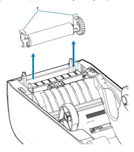
**4.** Slide the gear and the two bearings off the shaft of the platen roller.
