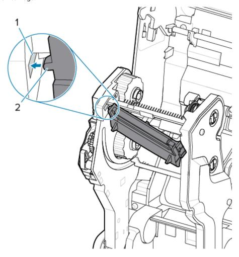
**8.** Push the right side of the printhead into the printer until the latch locks the right side of the printhead into the printer.
