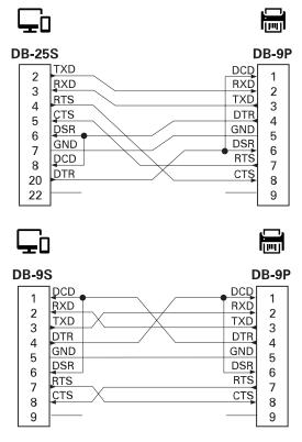
Interconnecting to DTE Devices – The printer is configured as data terminal equipment (DTE). To connect the printer to other DTE devices (such as the serial port of a personal computer), use an RS-232 null modem (crossover) cable.
