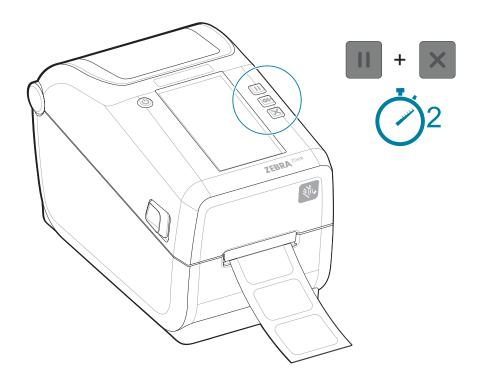
The printer will measure a few labels and adjust media sensing levels.
