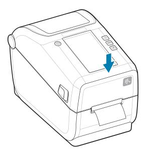
Calibrate the printer for the new media. The printer's sensors need to adjust to sense the label, the liner, and the distance between labels to operate properly.
