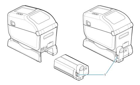
**3.** Attach the printer's power supply to the battery to wake up the battery from Shutdown Mode and begin its initial charge.
