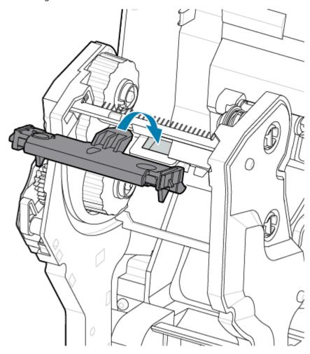
**7.** Insert the left side tab of the printhead assembly (2) into the recessed slot (1) on the left side of the ribbon carriage.
