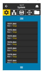
If ZBI programs have been downloaded to the printer, select one to run using this menu item. If no program exists on the printer, *NONE* is listed.
