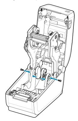
2. Place the adapter onto the roll holder.
