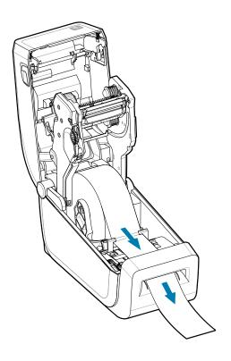
2. Close the printer. Press down until the cover snaps closed.
