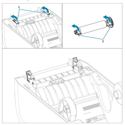
3. Lift the platen out of the printer's lower frame using the bearing arms (1).
