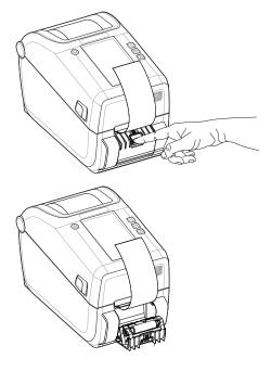
**3.** Insert the label liner between the dispenser door and the printer body.
