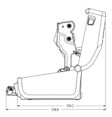
Figure 26 ZD611R Printer with the Media Cutter Option (dimensions in millimeters)
