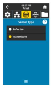
*Transmissive* (sees-through media and liner) — Used for gap/web sensing for common labels and continuous media. No tracking marks or notches on these media.
