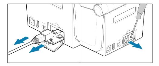
The Serial Port Module requires the use of fingers, a scribe, or a small flat-bladed screwdriver to pry the card out.
