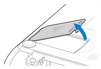
**7.** Align the antenna arm and lower the module into the printer body.
