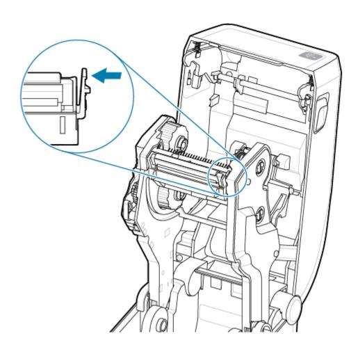
2. Swing the loose right side of the printhead out of the printer. Pull it to the right a little to get the left side of the printhead clear. Pull the printhead down and free of the ribbon carriage to gain access to its attached cables.
