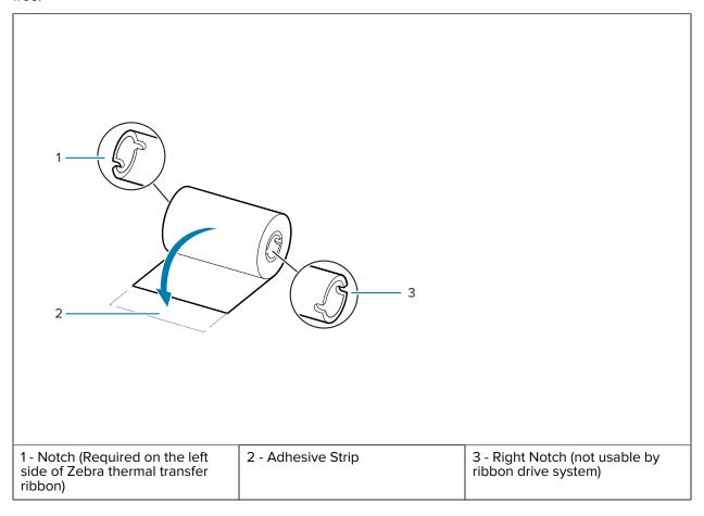
Verify that the ribbon and empty ribbon core have notches on the left side of the ribbon cores as shown above.
