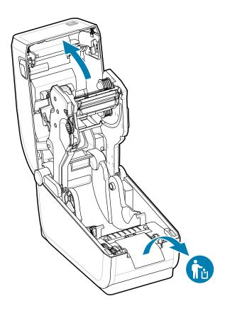
**3.** Inspect for any loose or damaged parts within the printer.
