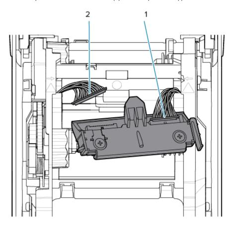
**6.** Insert the center tab on the printhead assembly into the center slot on the printhead mounting bracket in the ribbon carriage.
