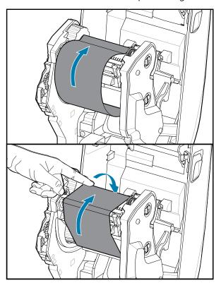
**3.** Attach the ribbon to the take-up core. Use the adhesive strip on new rolls; otherwise, use a thin strip of tape. Align the ribbon so that it will be taken straight onto the core.
