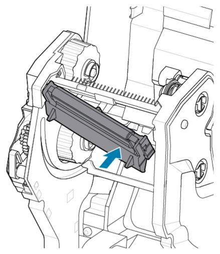
**9.** Verify that the printhead moves up and down freely when pressure is applied and remains locked when released.
