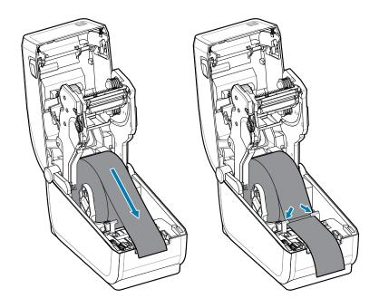
**6.** Flip the media up to access the sensor and the backside of the media.
