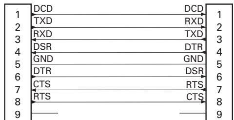
DB-9S Connector to DCE Device
