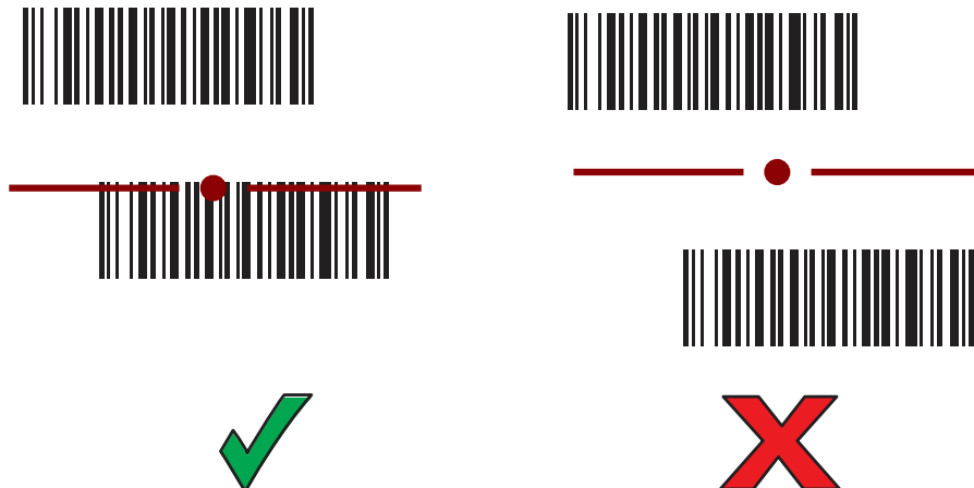
Figure 15 Pick List Mode with Multiple Barcodes - Extended Range
