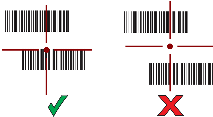
Figure 15 Pick List Mode with Multiple Barcodes - Extended Range
