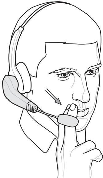
Figure 3-4 Adjust the Microphone Boom
