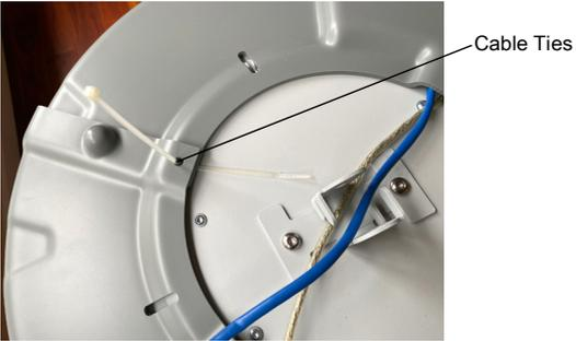
**NOTE** Cable ties must be applied on both sides.
