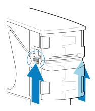
Use a screwdriver or similar object to push the media through the slot. Do not pull media out past the edge of the exit slot.
