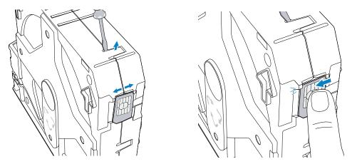
3. Secure the latch and ensure it is fully closed.
