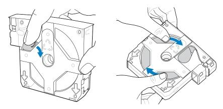
Pull the cartridge tabs up to open the media slot
