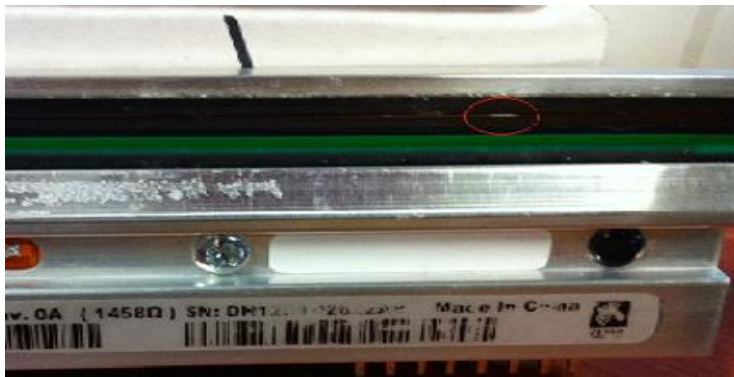
Physically damaged area
