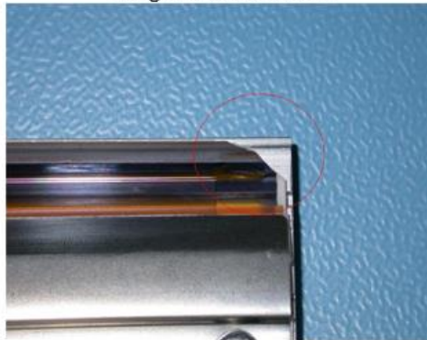
Chipped indication at right print head
