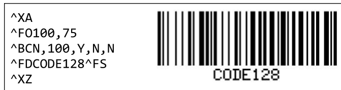
Figure 4 Subset B with Start Character
