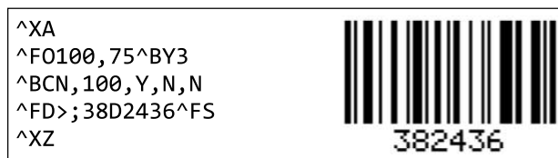
Figure 7 Subset C with Ignored Alpha Character
