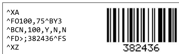
Figure 7 Subset C with Ignored Alpha Character
