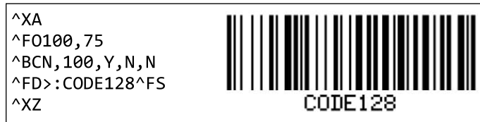
Figure 4 Subset B with Start Character
