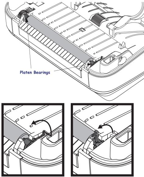
**3.** Lift the platen out of the printer's bottom frame.
