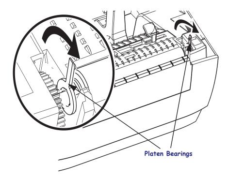
**3.** Lift the platen out of the printer's bottom frame.
